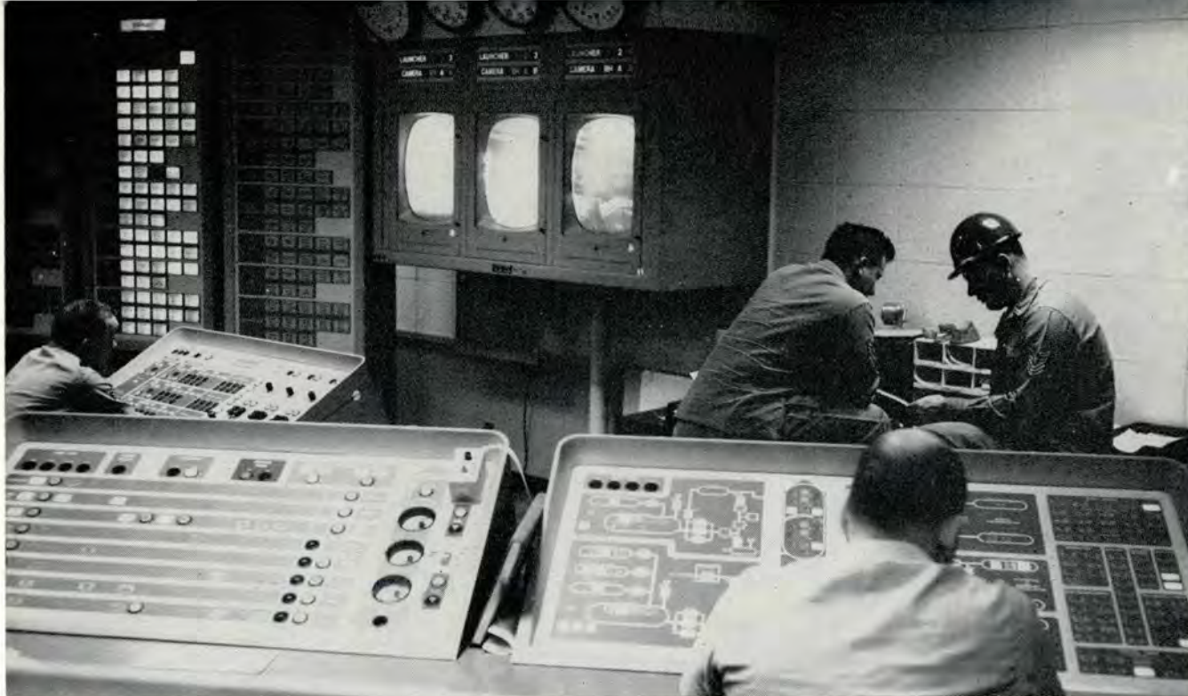
Thirteen technicians occupy this launch control center when a firing is imminent. Many pieces of launch control equipment are duplicated, assuring 100% back up capability in the event of a console malfunction. Visible are diagrams of various Atlas systems, all of which are monitored for countdown. The standby status panels to the left of the TV screens reflect the status of a sentry missile.
